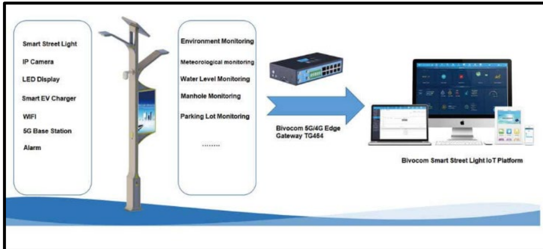
Smart Light Pole and its functions
